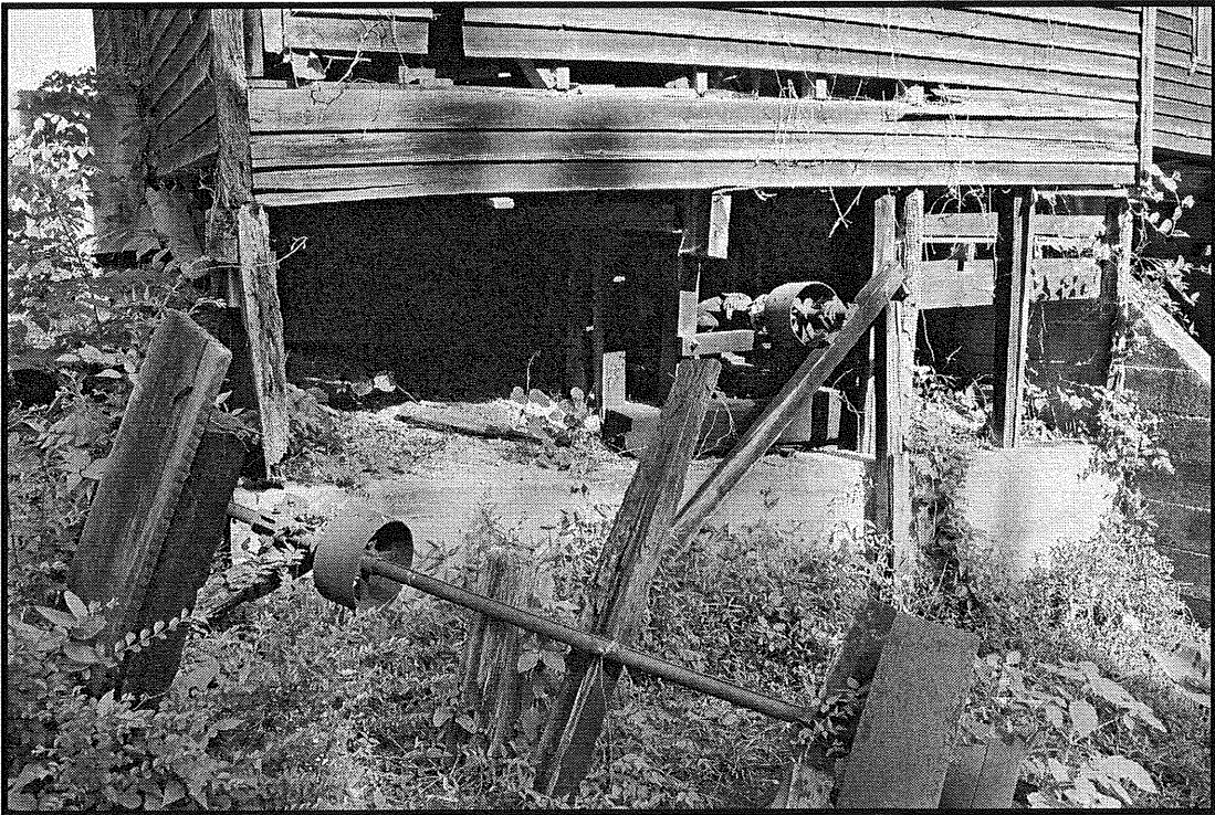
Plate 8: Parker's Mill – pulleys and shafts under and near southern block of mill
